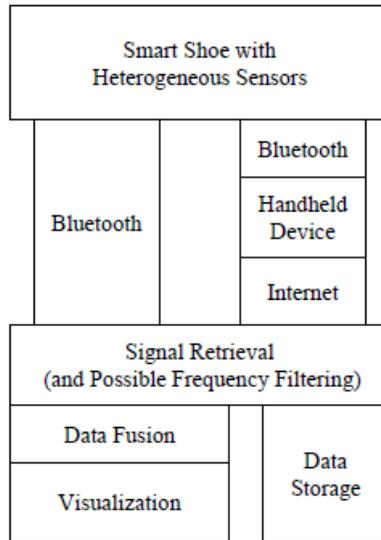
**Fig. 3.** Top-Level View of the System Interactions, from Sensor Data Collection to Wireless Transfer, to Visualization and Storage
