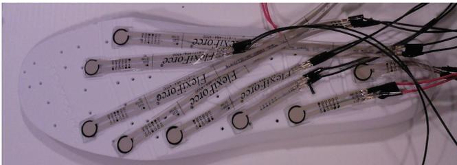
Fig. 2. Smart Shoe Insole Pressure Sensor Locations [14]
